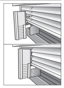
Clip the air separator, left and right of the partition, in the exhaust grille. Be sure that it clicks into place and guides the foam partition under the exhaust grille. All plumbing work should be carried out by a suitably qualified and competent person, in accordance with all applicable local and national regulations.
